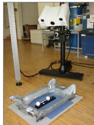
Fringe projection on automotive steel frame
